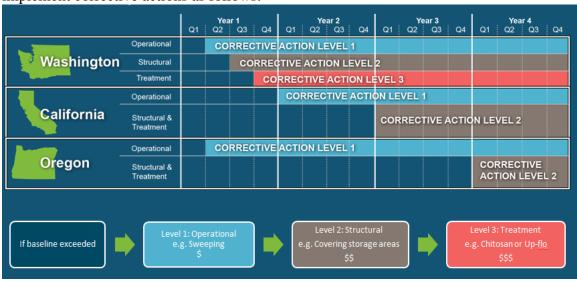
All of the Port's MTOs have triggered Level 3 Corrective Action. Level 3 Corrective Action consists of the design and construction of treatment systems to treat zinc, copper, and turbidity. These systems are often required to be sophisticated and are expensive. In addition to installing treatment systems, permittees must also install or enhance site-wide operational and structural source controls to achieve benchmarks.
